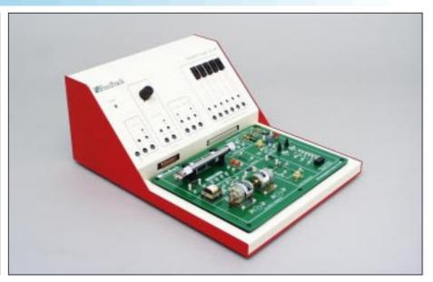
The Electromagnetism Trainer is designed as an introduction to the application of electromagnetic fields through the use of devices. It is a practical hands-on trainer where the elements in the system are presented on an open board in a clear and logical manner.
