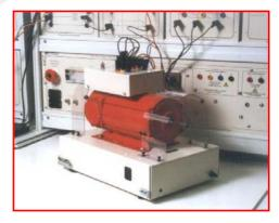
**Dissectible Machine:** - This provides over 50 different assemblies of dc, ac single phase and three phase machines. It is naturally more expensive than individual machines like those in our Industrial Machines range. It would be preferred when it is desirable for all students to carry out assignments on the same machine type at the same time. This operating
