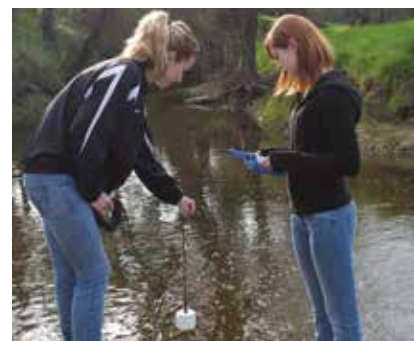
Study temperature vs. depth profiles of bodies of water – measure up to 10.5 m deep.
