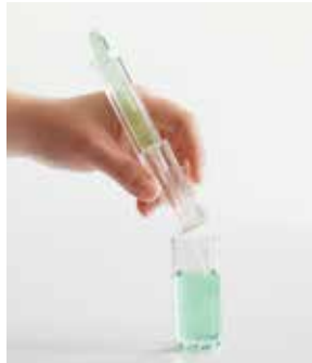
On final color change, turn titrator over and measure concentration using the built-in scale. That's it!
