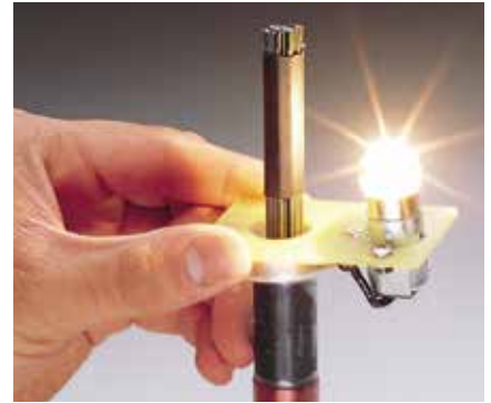
Lighting a bulb connected to a coil by induction; coil and bulb are included in Ring Launcher Accessories.
