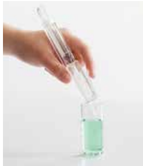
Begin titrating by gently squeezing the lever to draw in your sample.
