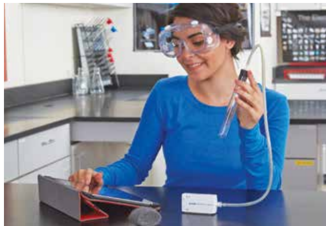
A test tube, piece of steel wool, and a Wireless Pressure Sensor are all you need to have your students calculate the amount of oxygen in the air.
