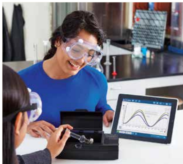
Determine the concentration of a sugar solution based on the optical rotation of plane polarized light.
