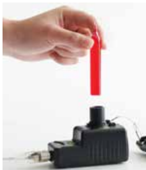
Place the vial in your Water Quality Colorimeter and read the results.
