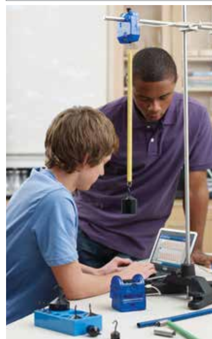
Combine with the Force Sensor to explore simple harmonic motion or Newton's Second Law.
