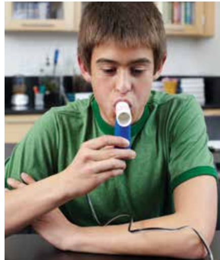
A student uses the spirometer to measure his lung volume. He observes the difference in the volume of his lungs when breathing normally vs. forced breathing.
