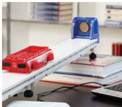
Integration of sensor and equipment makes changing the angle of incline a breeze.
