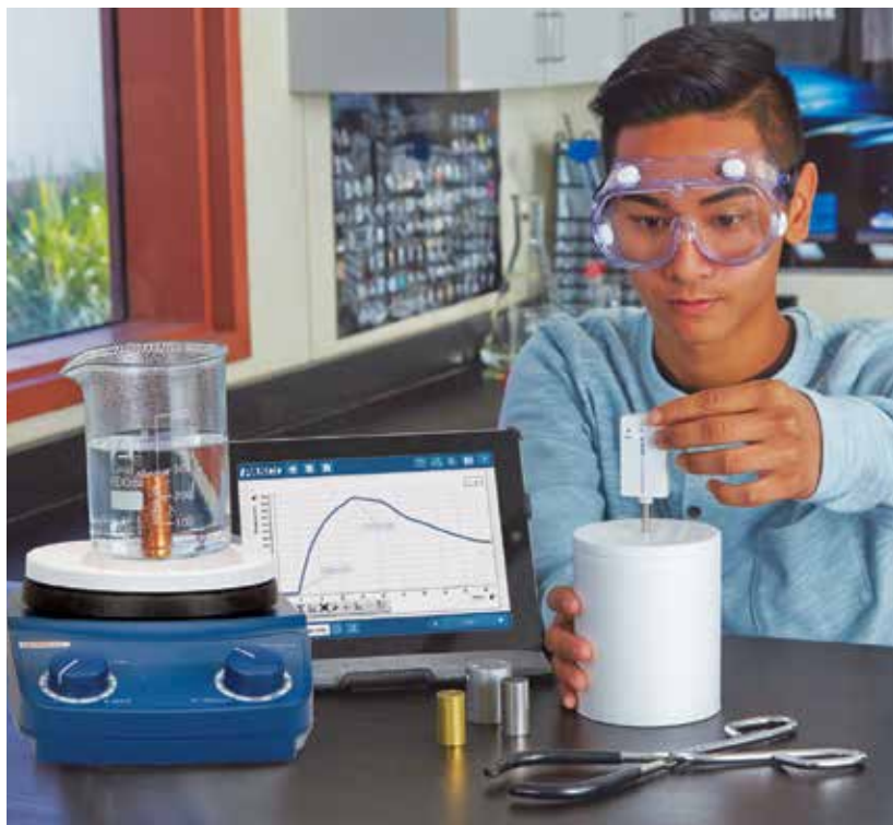
Use the change in temperature to determine specific heat capacity of a metal sample.
